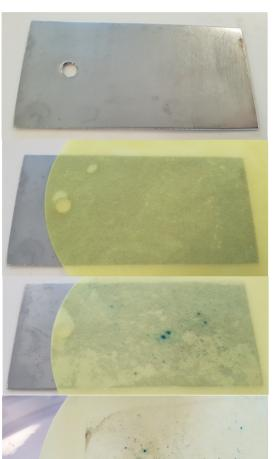
Test surface should be dust free, if needed, whipe with moist cloth before applying the Ferroxyl test paper
